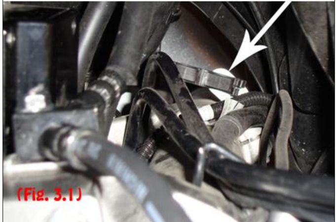
Looking straight down the fairing between the gauge cluster and the triple tree. This is an example of releasing the wire from the loom clamp.
